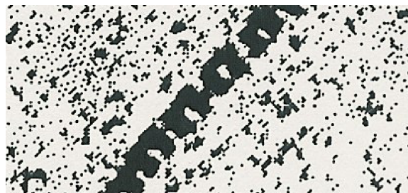
Fig. 6. Caterpillar structure of a monopole track (enlarged \cong 150 times).
